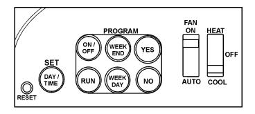
Most of the set up buttons and switches are located inside the front panel door. Gently pull the door down to access these.
