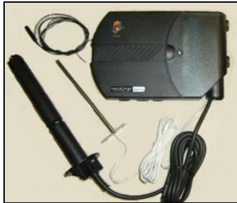
CASEY computer with attached air sensors
